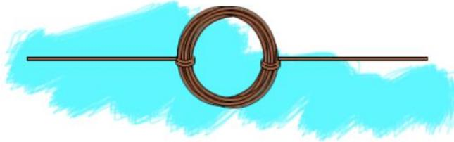
4. Using a small knife, remove the top half of the wire insulation on each free end of the coil. The exposed wire should be facing the same direction on both sides.
